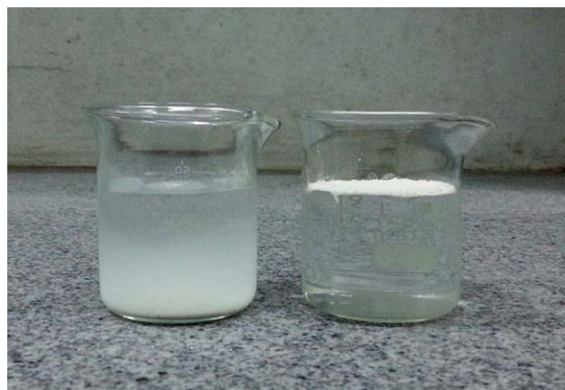
Figure 2. Hydrophobic test of unmodified \text{Sm}_2\text{O}_3 particles (left) and modified \text{Sm}_2\text{O}_3 particles (right). [Color figure can be viewed in the online issue, which is available at wileyonlinelibrary.com .]
